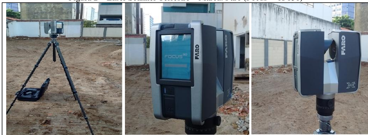
Figura 2 – Laser Scanner Terrestre – Marca: Faro (Focus 3D X 130)
